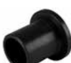
MOLDED FLANGE ADAPTOR SDR7 PE100 WATER / SU : 355 PSI GAS / GAZ : 125 PSI
