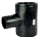
EF REDUCED TEE / EF İNEGAL TE SDR11 PE100 GAS / GAZ : 10 BAR WATER / SU : 16 BAR
