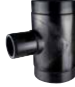
REDUCED TEE (SHORT) İNEGAL TE (KISA) SDR11 PE100 GAS/GAZ : 10 BAR WATER/SU : 16 BAR TYPE/TİP : SPIGOT
