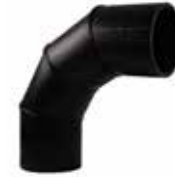
ELBOW (90°) SEGMENTED DİRSEK (90°) KONFEKSİYON SDR17 PE100 GAS/GAZ : 6 BAR WATER/SU : 10 BAR TYPE/TİP : SPIGOT
