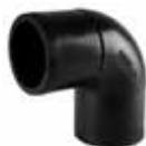
MOLDED ELBOW - 90° SDR9 PE100 WATER / SU : 255 PSI GAS / GAZ : 125 PSI
