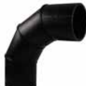
ELBOW (90°) SEGMENTED DİRSEK (90°) KONFEKSİYON SDR11 PE100 GAS/GAZ : 10 BAR WATER/SU : 16 BAR TYPE/TİP : SPIGOT
