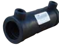
EF COUPLER (LONG) EF MANŞON (UZUN) SDR11 PE100 GAS / GAZ : 10 BAR WATER / SU : 16 BAR
