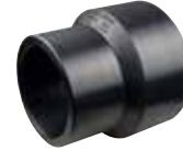
REDUCER (SHORT) REDÜKSİYON (KISA) SDR11 PE100 GAS/GAZ : 10BAR WATER/SU : 16 BAR TYPE/TİP : SPIGOT
